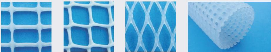
Extruded mesh is produced in rolls and made available in rolls or cut panels. From a spinning dye, threads are moulded over eachother into a tubular net. By cutting the net open, a flat net is created. Extrusion is a versatile process that allows production of nets varying from 1 mm to 300 mm mesh opening. Extruded meses are also produced in rigid tubular shape.
